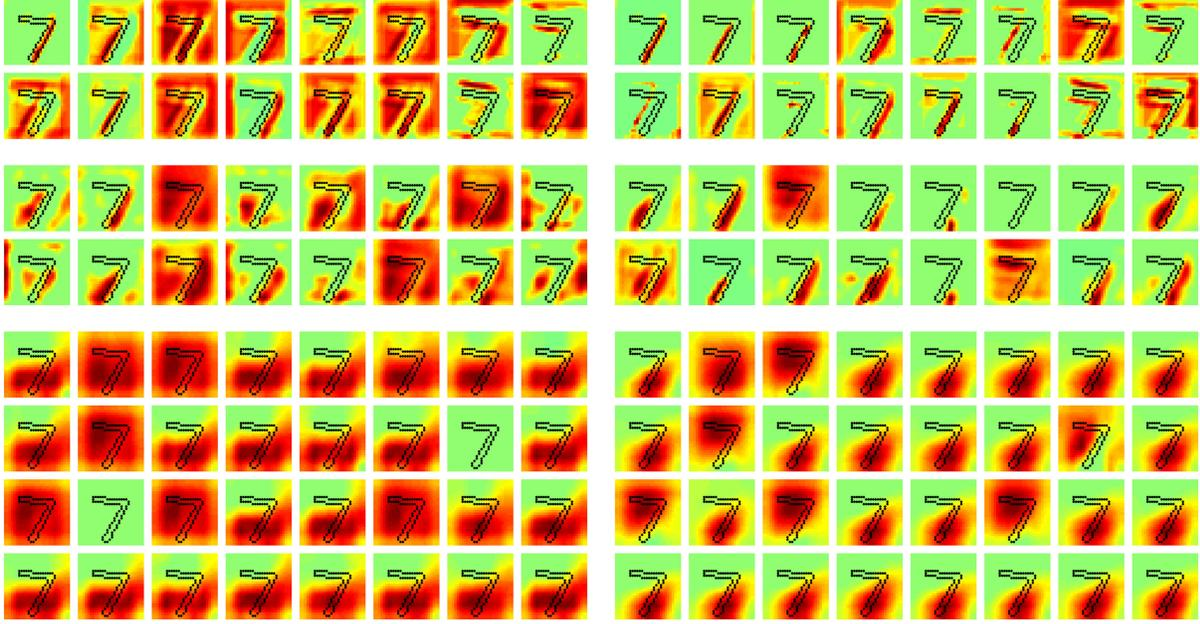
Figure 2. Activations of filters in the three convolution layers, using the “conventional training”(left) and the “proposed training”(right). From the top to the bottom, filter activations of the first, second, and third convolutional layers of the tested network.
